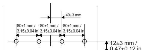
[4] Puncher unit-P1 (4-Hole (SWD))
